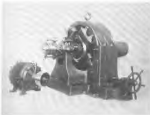
Figure 4 Synchronous generator and induction motor from the time of Nikola Tesla
