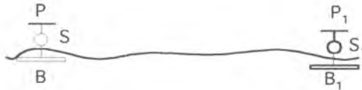
Fig.5. Tesla's proposition from 1893: S - h.f. generator; B- ground plate; P-elevated plate (antenna). Receiver is tuned to the transmitter frequency
